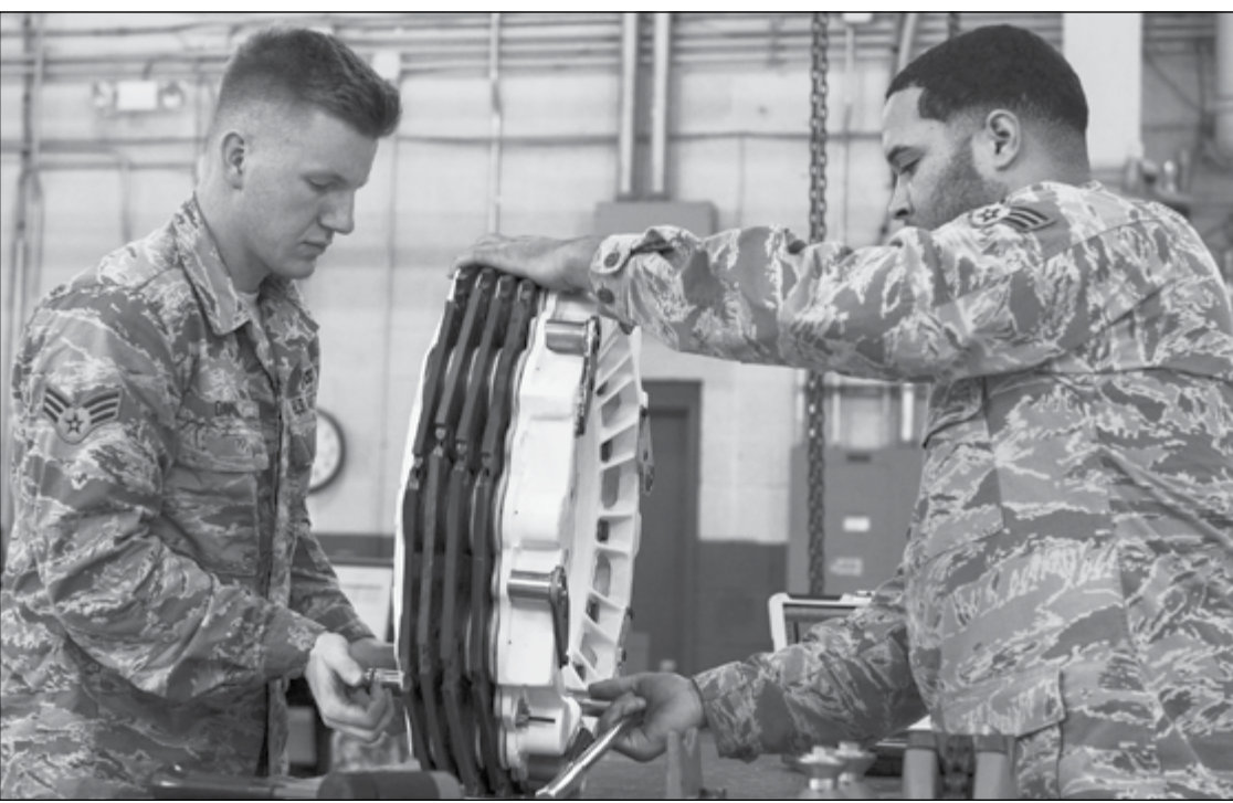
U.S. Air Force photo/Airman 1st Class Tessa B. Cormick Senior Airmen Taylor Davis and Nathan Pennington, 2nd Maintenance Squadron bomber hydraulic centralized repair facility journeymen, work together Oct. 23 to ratchet a bolt into a brake for a B-52 Stratofortress at Barksdale Air Force Base, La.
